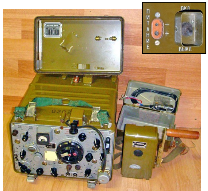
R-131 with Morse key attached and Z-348m hand cranked generator for charging the internal batteries. Inset: on-off switch and charging sockets located on top at the far end.
