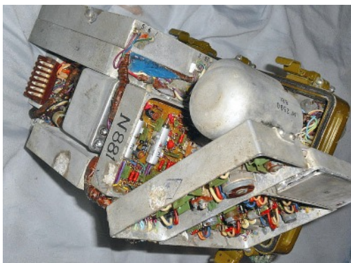
Internal view of R-131 showing its modular construction (left).
