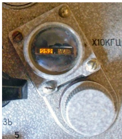
Dial reading was in kHz x10 indicated on a projection scale with lens (here set to 2520kHz).
